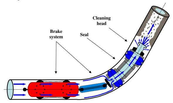
All units have openings that allow the entire fluid flow through the pipeline to bypass. The brake unit ensures that the HAPP is held back against the fluid flow in the pipeline. The fluid pushes against the following seal unit, which channels it into the openings of the cleaning head. Seal unit and cleaning head pose a flow restriction resulting in a pressure difference across HAPP. The fluid is accelerated in the cleaning head's nozzles creating extremely
